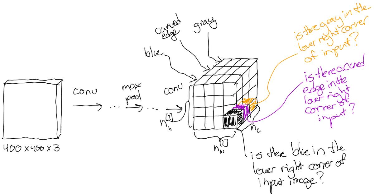
"Unroll" the 3d array of activation outputs into a matrix
