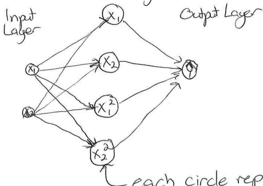
~~Neuron~~ each circle represents an intermediate quantity calculated by a "unit" or "neuron", and used as an input to the next layer.
